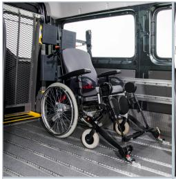
The wheelchair enters the vehicle via lift. AMF-Bruns PROTEKTOR system for wheelchair and occupant restraint.
